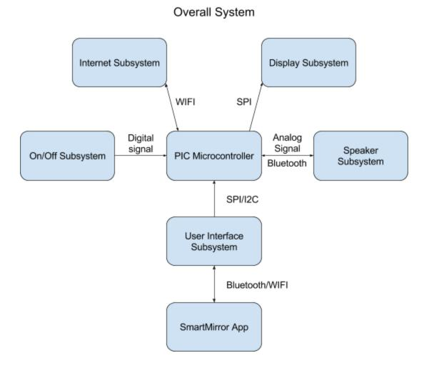
On/Off Subsystem: This subsystem will deal with determining whether someone is in front of the mirror or not. Using a PIR sensor, it will intelligently turn/keep the mirror on or turn/keep the mirror off.
